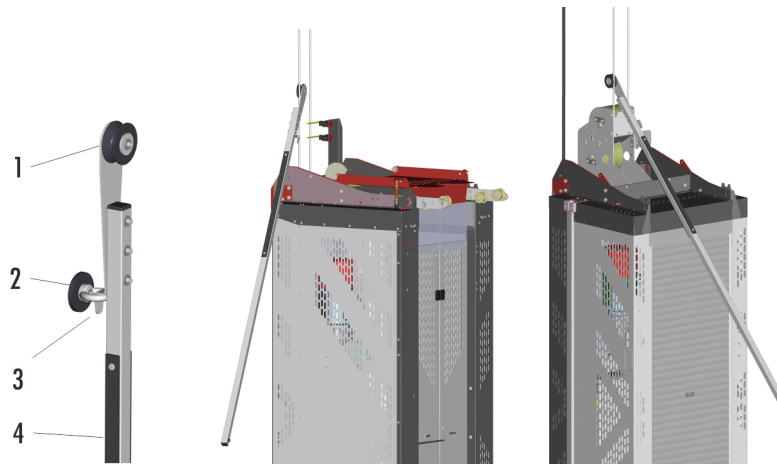
Fig. 12: Rope pull rod with TOPlift L and GLOBALift R (f.l.)
